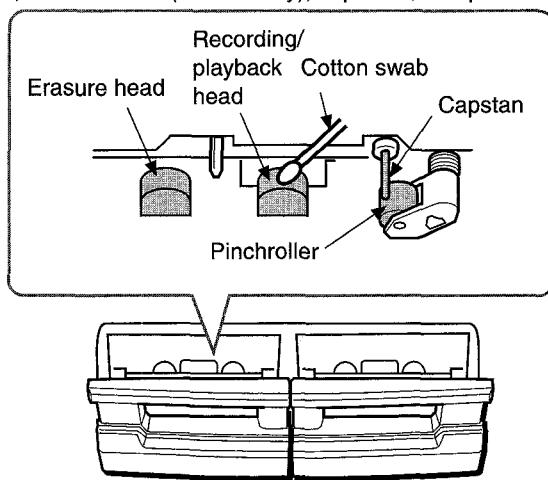
After cleaning the heads and tape paths with a liquid head cleaning cassette or a moistened swab, wait until the cleaned parts are completely dry before inserting the tapes.
